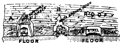
FIG. 218.—Section of pillars and stalls.
